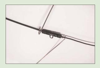
This is the long awaited solution for inspectors' request to get connectors and cables out of water and snow on rooftops. Solar Snake Charmer snaps into place under the panel to carry connectors safely and securely at the rear of the panel.
